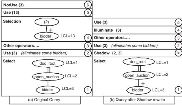
**Figure 12: Shadow/Illuminate rewriting procedure.** This generic example is indicative of how the procedure is performed. Note how the APT for Selection 1 has been replaced by an APT using an “+” annotated edge followed by the Shadow 1a operator. Selection 4 is replaced by Illuminate 4. We have eliminated redundant access to the database.
