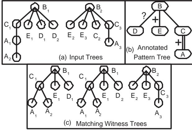
**Figure 4: A sample match for an Annotated Pattern Tree. Any edge without an explicit annotation implies the default “-”. The double-edged lines represent an ancestor - descendant relationship. Note how the APT addresses heterogeneity on both dimensions (height and width) using variations of annotated edges.**
