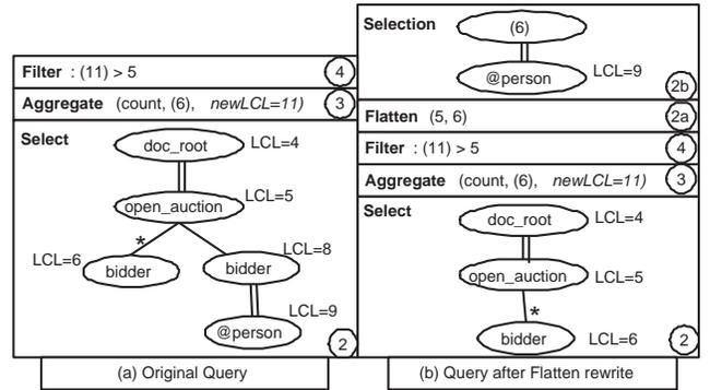
Figure 10: Flatten Rewrite for Query Q1. Please note how *Selection 2* from the original plan has been replaced by *Selection 2* with a sub-tree of the original pattern tree containing only the path with “\*”. *Flatten 2a* has been added after the aggregate has used the *bidder* nodes. Then *selection 2b* extends the *bidder* elements with *person*. The right block substitutes the left block eliminating redundant tree matches.
