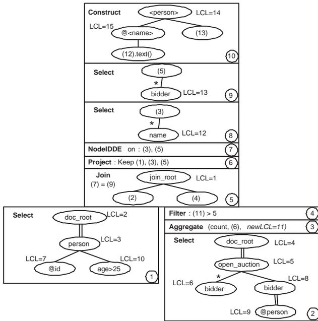
**Figure 7: Algebraic Tree for Query Q1.** Order of evaluation is bottom-up. Each box represents an operator. Each APT edge has the matching specification marked next to it, except for the default “.” which is omitted for clarity. (ad) relationships use double edges. The LCLs assigned to each class are shown next to the corresponding APT node.
