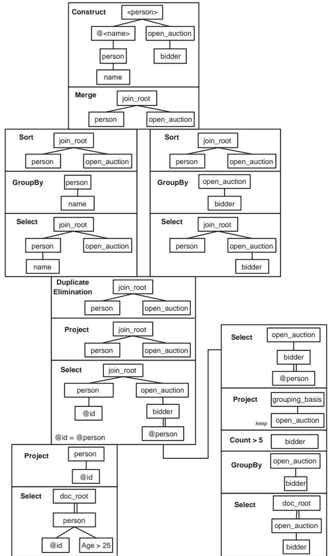
Figure 2: An Algebraic Plan of Example Query Q1. The evaluation is bottom up. For clarity, we have presented this as an evaluation “plan”, and pictured the pattern tree used by each operator, rather than writing out a complex formal expression. Many details have been suppressed. The operators used are borrowed from TAX, we define the TLC variants in section 2.3.
